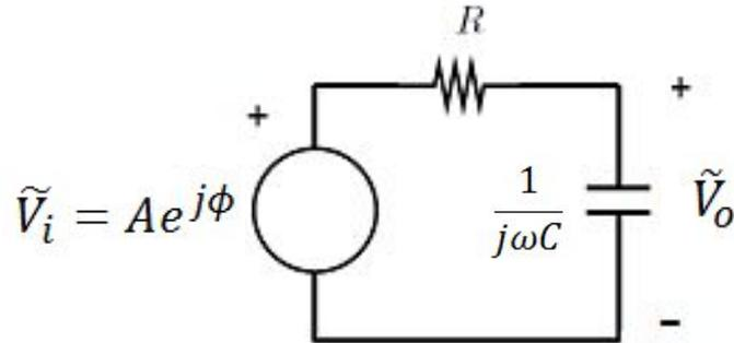
$$v_o(t) = \text{Re}(\tilde{V}_o e^{j\omega t}) = \text{Re}\left(\frac{1}{1 + j\omega RC} \tilde{V}_i e^{j\omega t}\right) = \text{Re}\left(\frac{A}{1 + j\omega RC} e^{j(\omega t + \phi)}\right)$$
