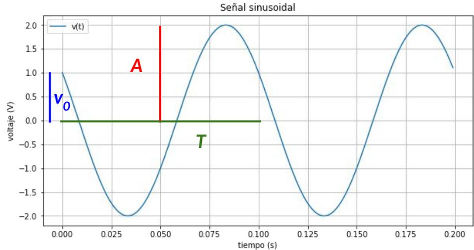
$$v_{i,0} = v_i(0) = A \cos(\phi) \rightarrow \phi = \arccos\left(\frac{v_{i,0}}{A}\right) + \pi k, k \in \mathbb{Z}$$
