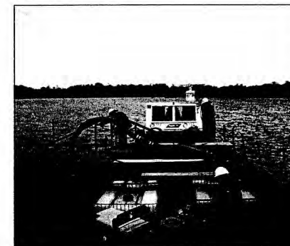
Sediment in Ranworth Broad being treated with iron salts.
