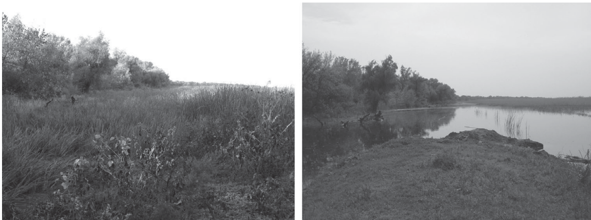
FIGURE 13.5 Removing artificial levees will also restore wetlands. (left) Prior to dike removal. (right) After removing some 6 km of dikes, natural flood regimes were restored and in 2004 the Danube River flowed freely over Tataru Island. (Courtesy World Wildlife Fund.) (See also color plate.)
