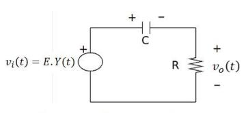
$$\frac{d}{dt}v_o(t) + \frac{1}{RC}v_o(t) = \frac{d}{dt}v_i(t)$$
