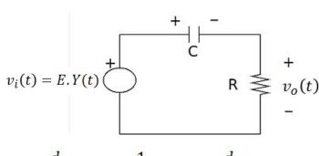
$$\frac{d}{dt}v_o(t) + \frac{1}{RC}v_o(t) = \frac{d}{dt}v_i(t)$$
