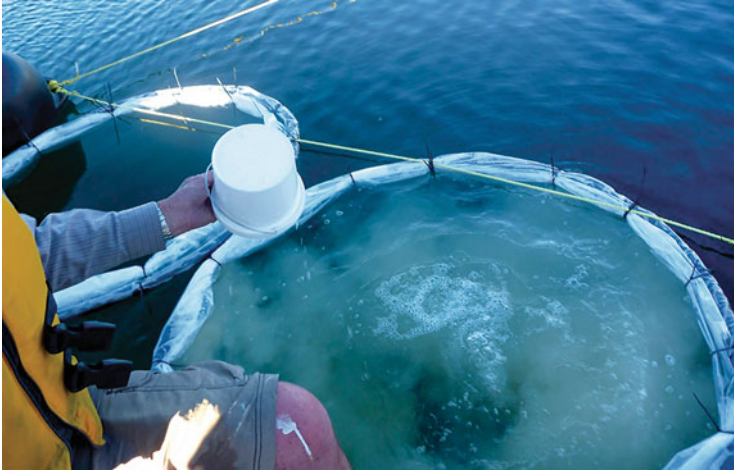
Fig. 7.12 Floc formation after dosing at a rate of 70 \text{ g alum m}^{-2} into a 10-m-deep mesocosm in a high alkalinity lake (alkalinity >400 \text{ gEq} ) [photo by C. Hickey, NIWA]
