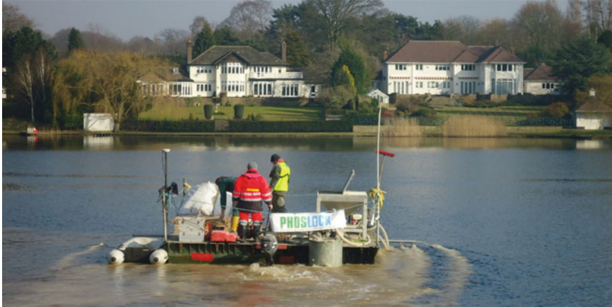
Fig. 7.3 Geo-engineering trial of a modified lanthanum bentonite product called ‘Phoslock’ at Mere Mere, UK. Image courtesy of Bryan Spears, Centre for Ecology & Hydrology, UK
