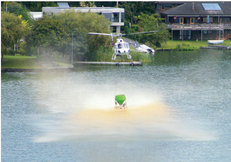
Fig. 7.18 Application of Aqual-P ® <1 mm slurry by helicopter from a monsoon bucket fitted with a fertiliser spreader. The helicopter position was controlled using GPS navigation [photo: Graham Timpany, NIWA]
