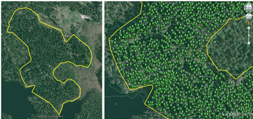
Fig. 7.7 Aerial photo of the harvest area (left) and identification of individual trees of a part of the area based on aerial laser scanning (right)
