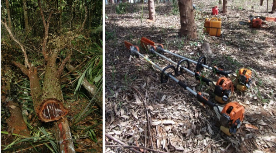
Fig. 11 Risky delimiting of branches in native forests with the help of a chainsaw ( left ) and in a planted forest with the help of small chainsaws with extension for improved ergonomic position of the workers
