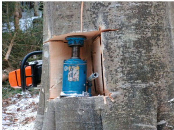
Fig. 10 Directional felling to avoid damages on remaining trees or improve safety of forest workers
