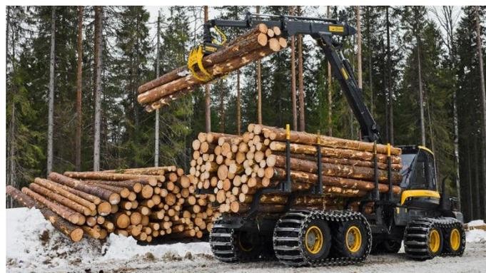
*Figura 18 – Forwarder descargando madera.*
