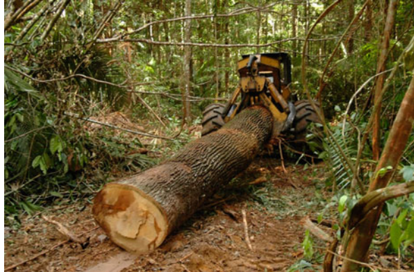
Fig. 14 Skidding operation in native forests with help of a grapple skidder (Source Leif Nutto)
