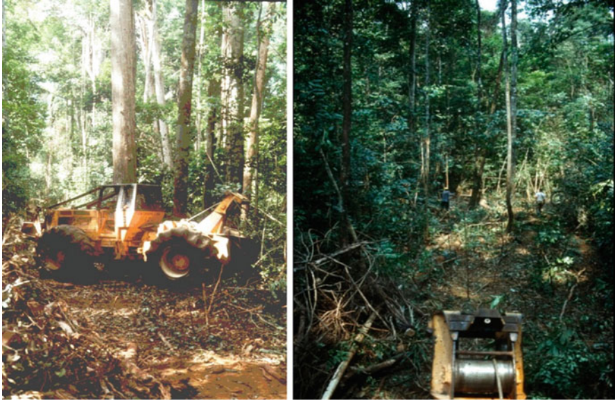
Fig. 15 Skidder with winch ( left ) and winching process ( right ) (Source: Grammel 1995)
