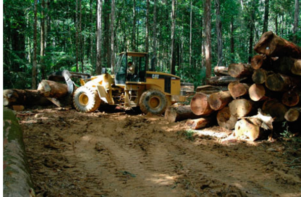
Fig. 17 Piling of logs at a landing zone beside a secondary road using a wheeled front-end loader (Source: Leif Nutto)
