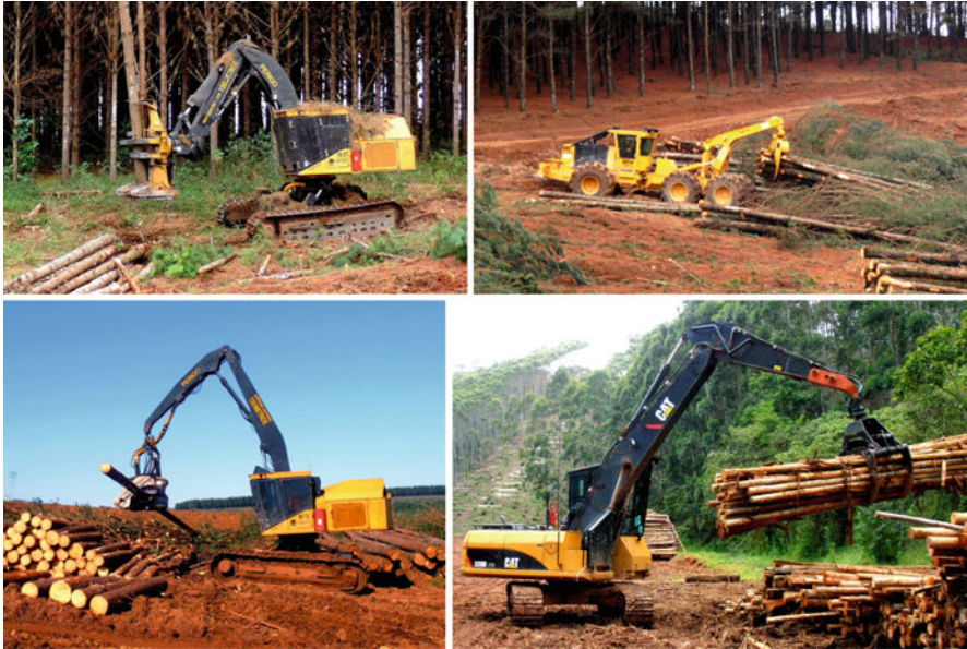
Fig. 6 Feller buncher ( up, left ), skidder ( up, right ), processor ( down, left ), and log loader ( down, right ) are the main machines used in full-tree systems (Source: Gustavo Castro)
