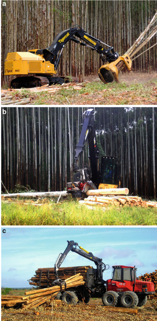
Fig. 20 Cut-to-length system using a feller buncher (a), a harvester working as a processor (b), and a forwarder for wood extraction (c) (Source: Gustavo Castro)
