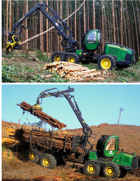
Fig. 4 Harvester and forwarder as the main machines used in the cut-to-length system (Source: Gustavo Castro)
