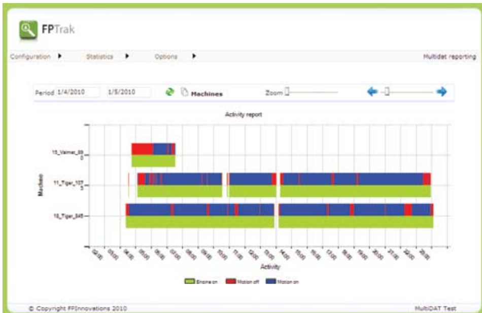
Figure 14: FPDat website reporting (FPTrak). Example of a pre-defined report produced from data uploaded to the FPTrak online server
