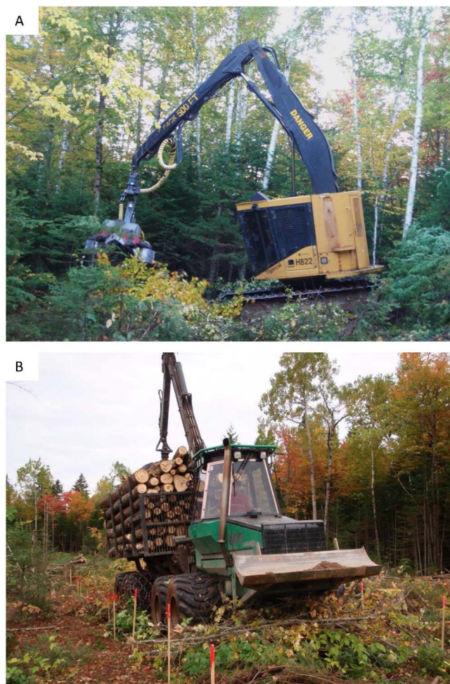
Fig. 2. A. Tigercat H822 single-grip harvester and B. Logset 8F forwarder used in the study.
