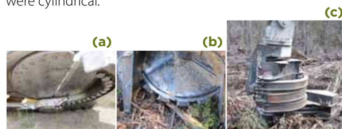
Figure 1. Feller-buncher head types (a) shear; (b) hotsaw; (c) chainsaw
