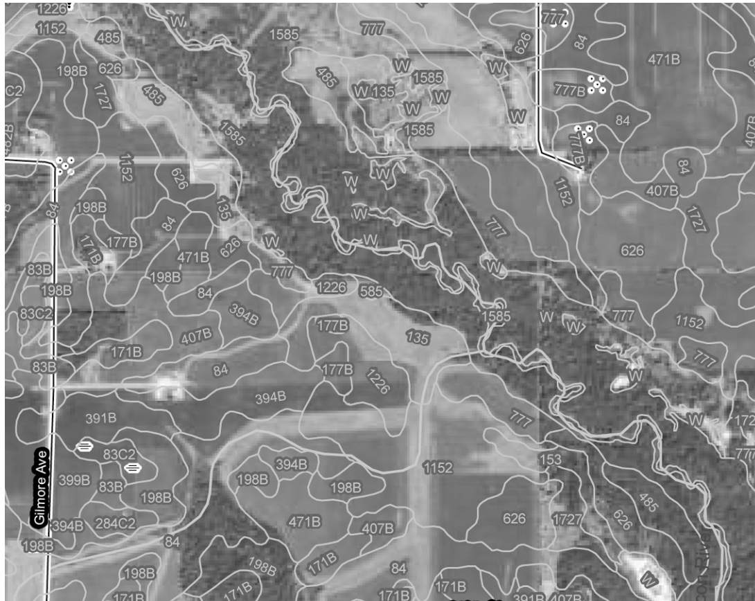
Figure 6.7 The relation of soils to topography is apparent in this map of local soil series in an area of Chickasaw County, Iowa from the web soil survey. (Courtesy of USDA Natural Resources Conservation Service.)
