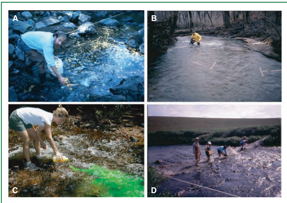
FIGURE 13.2 Photographs of (A) Ginkgo biloba leaf release into an Oregon stream, (B) wood dowel collection following release in a Michigan stream at high flow, (C) fluorescein dye release into an Indiana stream, and (D) beach seine stretched across the channel of a northern Alaska stream (anchored to the bottom with rocks) for capturing unretained leaves. (Photos by G. Lamberti.)
