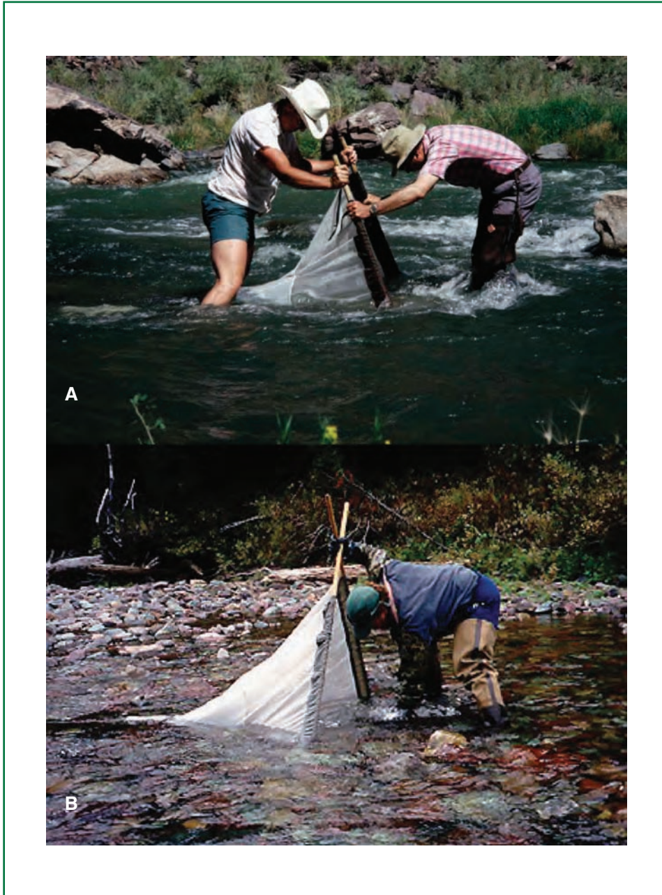
FIGURE 20.3 Field pictures of the Stanford-Hauer kicknet being used by (A) two persons and (B) by a single person. Note the extended net and bucket end of the kicknet sampler.
