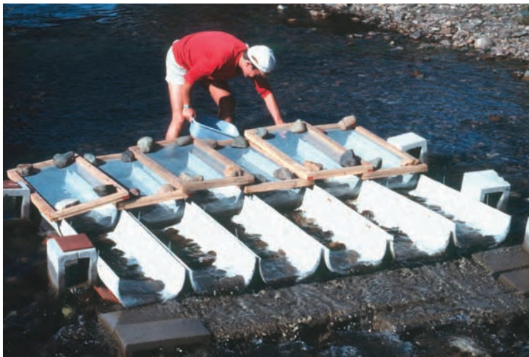
FIGURE 23.3 Photograph of 12 large, submersed PVC enclosures (dimensions: 103 cm L × 32.5 cm D) used to study grazing tadpoles in high-gradient streams near Mount St. Helens, Washington, USA. Enclosures contain algal-covered stream cobbles that are used both as grazing substrata for tadpoles and as ballasts for enclosures in fast riffles. Coarse mesh covers used to isolate and protect animals are shown in the 6 enclosures in the upper part of photograph. Direction of flow is from upper left to lower right of photograph (see Feminella and Hawkins 1994).
