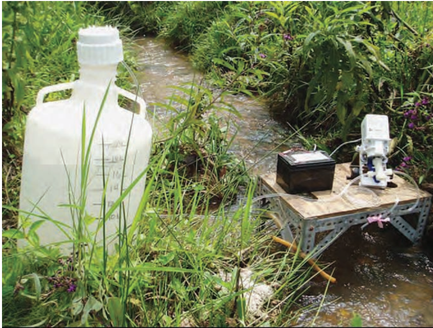
FIGURE 8.1 Field setup for a solute release. This setup was used in a small agricultural stream in North Carolina. The 20-L carboy contained the mixed release solution, and the small table in the stream was used to stabilize the metering pump and battery. The solution was dripped into the center of the stream where the pink ribbon is tied to the hose. Photo by Rob Payn.
