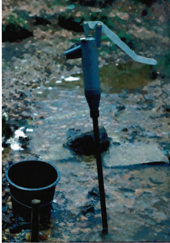
FIGURE 19.2 Bou-Rouch pump for qualitatively sampling meiofauna from streambeds that are hard to penetrate with corers. The pump stand has a perforated lower hollow column into which water and associated fauna can seep and from which water is then pumped up and sieved. (Photo credit: Simon Rundle.)
