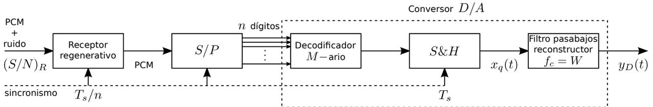
Figura 8: Receptor PCM.
