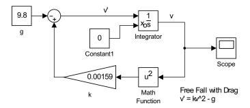
Figure 2.9: Model for free fall with drag as described by  $\dot{v} = kv^2 - g$ .
