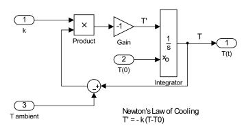
Figure 2.5: Creating a subsystem for the Newton's Law of Cooling model.
