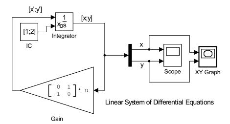
Figure 5.4: Linear system using matrix operation.
