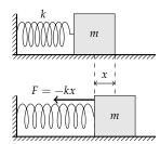
Figure 3.6: A simple harmonic oscillator consists of a mass, *m*, attached to a spring with spring constant, *k*.
