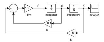
Figure 3.9: A model for damped simple harmonic motion,  $m\ddot{x} + b\dot{x} + kx = 0$ .
