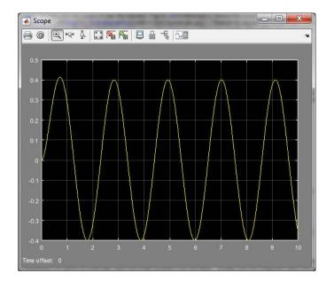
Figure 1.16: **Scope** plot of the solution of  $\frac{dx}{dt} = 2\sin 3t - 4x$ , x(0) = 0, with **Refine Factor**= 10.
