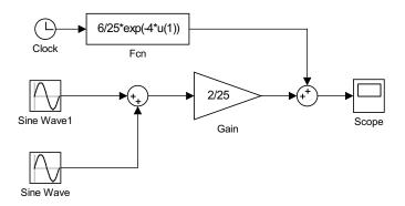
Figure 1.24: Model for plotting the exact solution (1.8) of the initial value problem (1.6).
