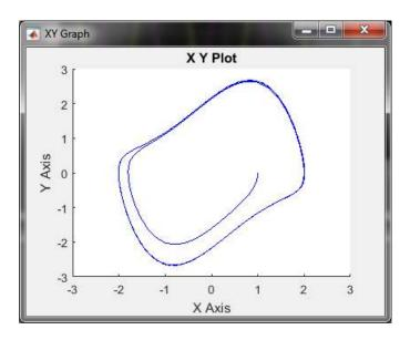
Figure 5.9: Phase plane plot for the van der Pol equation.
