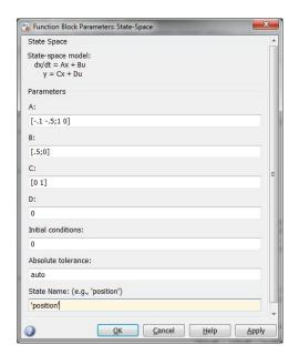
Figure 4.3: State space block parameters.
