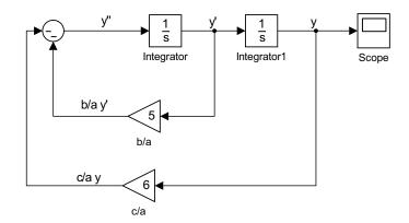
Figure 3.3: Model for the second order constant coefficient ODE y'' + 5y' + 6y = 0.
