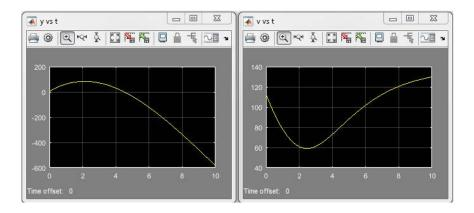
Figure 3.20: Output of the Scope Blocks for the projectile motion model for position and velocity vs time.
