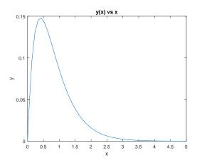
Figure 3.4: Solution plot for the initial value problem y'' + 5y' + 6y = 0, y(0) = 0, y'(0) = 1 using Simulink.
