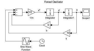
Figure 3.12: A model for forced simple harmonic motion,  $m\ddot{x} + kx = \sin \omega t$ .
