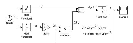
Figure 1.22: Linear first order differential equation model.
