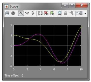
Figure 4.4: Solution to the forced, damped harmonic oscillator problem with initial conditions set to o or [0;1].
