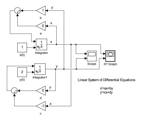
Figure 5.1: Linear system using two integrators.
