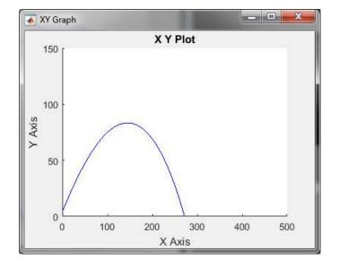
Figure 3.21: Output of the XY Graph block for the projectile motion model showing vertical position vs horizontal position.
