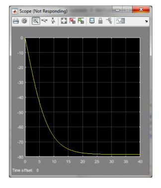
Figure 2.10: Solution for free fall with drag with k = 0.00159 starting from rest.
