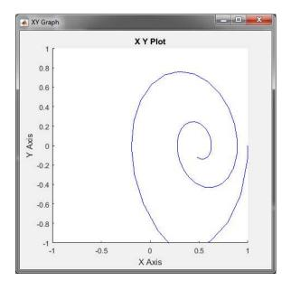
Figure 3.18: XY Graph output for the solution of the forced, damped, harmonic oscillator model.
