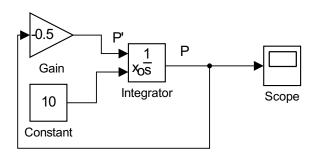
Figure 2.1: Simulink model for exponential growth and decay. The initial value, P(0) = 10, is set in the **Constant** block and k = -0.5 is set in the **Gain**.
