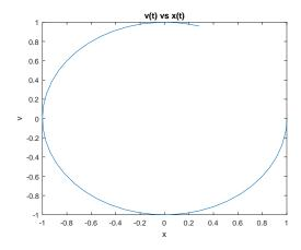
Figure 3.33: Phase plot for the simple harmonic oscillator.
