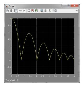
Figure 3.26: Output from the bouncing ball model showing plot of height vs time.
