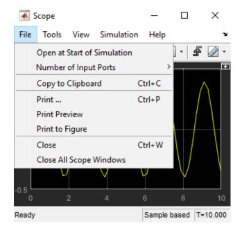
Figure 1.28: Scope plot showing File menu where one can Print to Figure.
