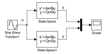
Figure 4.5: The use of the State Space Block dispaying a Sine Wave input and output to a **Scope**. The **Mux** block (from Signal Routing) is used to feed solutions from two systems using different initial conditions.
