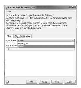
Figure 1.9: Block Parameters for the Sum control. In many cases it is best to also select the rectangular shape over the default round shape.
