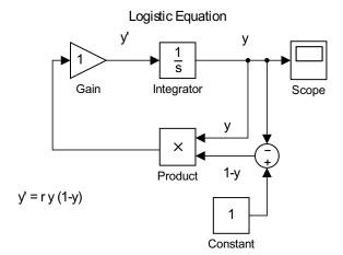
Figure 2.14: Simulink model for the logistic equation, y' = ry(1 - y).
