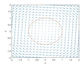
Figure 3.34: Phase plot for the simple harmonic oscillator.
