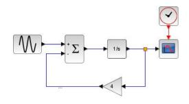
Figure 1.41: The Xcos model for solving the first order ODE  $\frac{dx}{dt} = 2\sin 3t - 4x$ .
