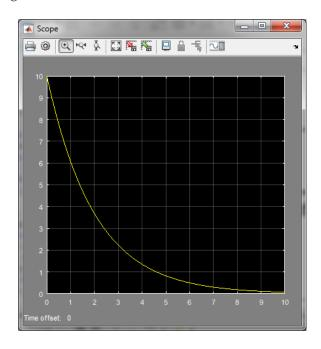
Figure 2.2: Solution for the exponential decay with P(0) = 10 and k = -0.5. The simulation time was set at 10.
