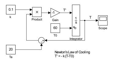
Figure 2.3: Simulation model for Newton's Law of Cooling,  $T' = -k(T - T_a)$ , T(0) = T0. Here we set  $k = 0.1 \text{ s}^{-1}$ ,  $T_a = 20^{\circ}\text{C}$ , and  $T_0 = 60^{\circ}\text{C}$ .
