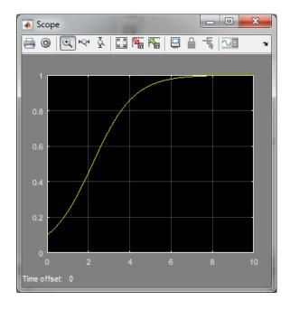
Figure 2.15: Solution of the logistic equation, y' = ry(1 - y), with r = 1 and y(0) = 0.1.
