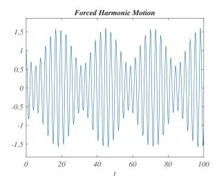
Figure 3.14: The analytic solution for the forced harmonic oscillator example.
