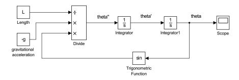
We enter the parameters in the system using variables instead of particular constants. These parameters are introduced in a MATLAB m-file. The constants are **L**, **g**, and initial conditions **thetao** and **vo** in the **Integrator** blocks. Save this model as **pend.mdl**.
