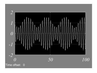
Figure 3.13: Output for the solution of the forced simple harmonic oscillator model.
