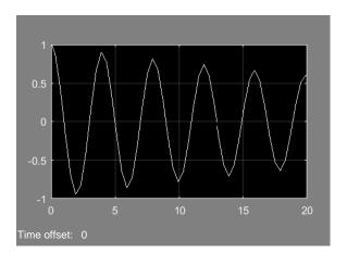
Figure 3.10: Output for the solution of the damped harmonic oscillator model.
