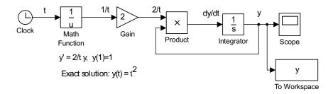
Figure 1.25: Adding To Workspace block for sending output to MATLAB.
