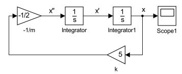
The output on the scope is shown in Figure 3.8 for  $t \in [0, 10]$ . Solving the initial value problem we find that  $x(t) = \cos \omega_0 t$ , where
