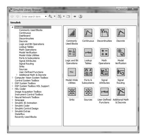
Figure 1.5: The Simulink Library Browser. This is where various blocks can be found for constructing models. [As seen in MATLAB 2015a.]
