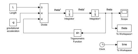
Figure 3.29: Nonlinear pendulum model with To Workspace blocks added to output  $\theta(t)$  and t.
