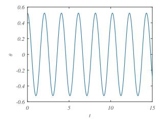
Figure 3.30: Plot of solution,  $\theta(t)$  vs t, to the nonlinear pendulum model.
