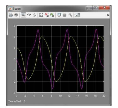
Figure 5.8: Solution plot for the van der Pol equation.
