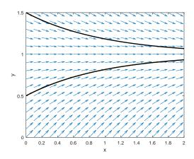
Figure 1.47: A direction field produced using MATLAB's quiver function for y' = 1 - y with solution curves added.
