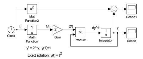
Figure 1.20: First order separable differential equation model with extra blocks to plot the difference between the numerical and exact solution,  $y(t) - t^2$ , for Equation (1.2).
