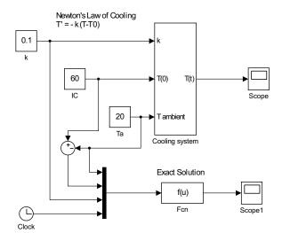
Figure 2.8: Model of Newton's Law of Cooling,  $T' = -k(T - T_a)$ , T(0) = T0, using the subsystem feature.
