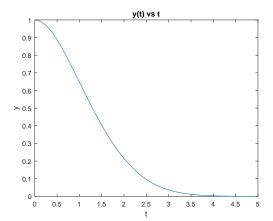
Figure 1.45: A plot of the solution of  $\frac{dy}{dt} = -\frac{yt}{\sqrt{2-y^2}}, \quad y(0) = 1, \text{ found using}$ MATLAB's **ode45** command.
