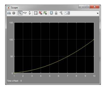
Figure 1.19: Scope plot of the solution of initial value problem (1.2),  $\frac{dy}{dt} = \frac{2}{t}y$ , where y(1) = 1.
