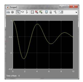
Figure 3.16: Forced, damped oscillator.
