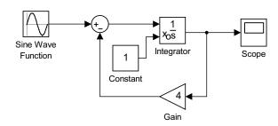
Figure 1.17: Connections for the First Order ODE model for  $\frac{dx}{dt} = 2 \sin 3t - 4x$  showing how to provide an external initial value.
