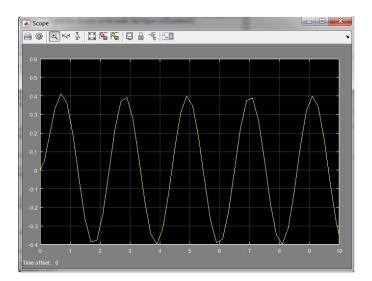
Figure 1.13: Scope plot of the solution of  $\frac{dx}{dt} = 2\sin 3t - 4x$ , x(0) = 0, with Refine Factor = 1.
