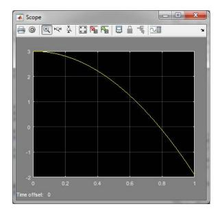
Figure 3.23: Height vs time Scope plot for the free fall model.
