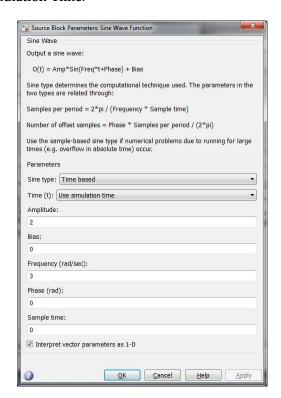
Figure 1.10: Parameters for the Sine Wave block. Select the amplitude and frequency desired.
