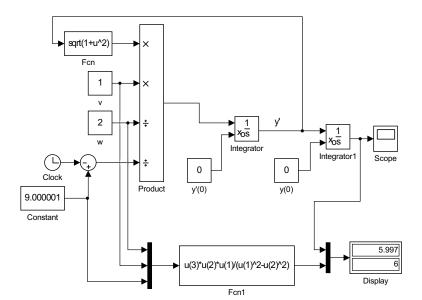
Figure 2.12: Model for the pursuit curve,  $(a - x)y'' = \frac{v}{w}\sqrt{1 + [y'(x)]^2}$ , y(0) = 0, y'(0) = 0, for w = 2 and
