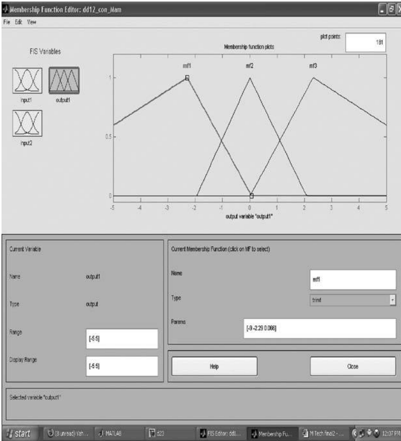
FIGURE 9.53 Membership function plot of output of fuzzy controller.
