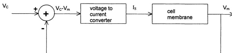
*Figure 10-5.* Block schematic of the experiment for voltage clamping a membrane.
