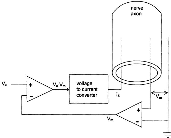
Figure 10-6. Schematic of the voltage clamp experiment.
