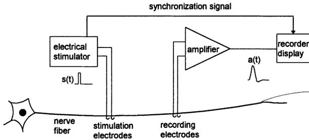
*Figure 10-1.* Recording a nerve action potential. The stimulus  $s(t)$  initiates an action potential which is observed as  $a(t)$ .
