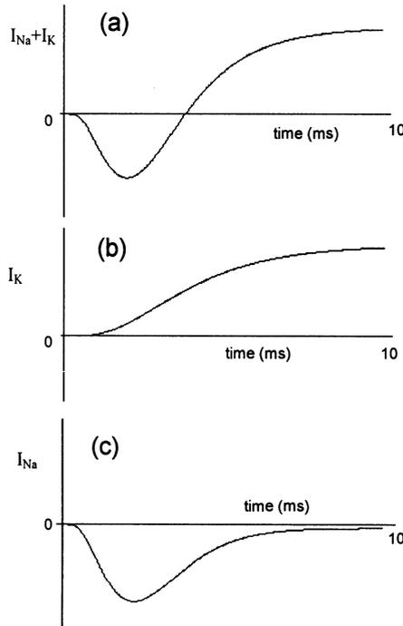
*Figure 10-7.* Voltage clamped membrane currents. (a) potassium and sodium current, (b) potassium current, (c) sodium current calculated as the difference of the first two. (Adapted from A.L.Hodgkin and A.F.Huxley, A quantitative description of membrane current and its application to conduction and excitation in nerve, *J.Physiol.* **117**: 500-544, 1972.)
