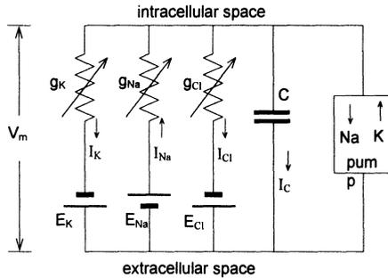
*Figure 10-3.* Electrical equivalent of a nerve membrane.
