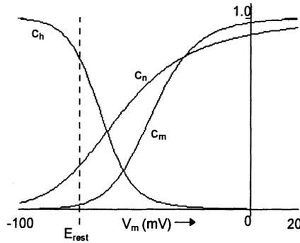
Figure 10-11. The amplitude constants plotted against the membrane voltage.
