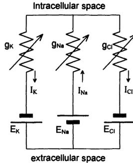
Figure 10-2. Electrical equivalent of ionic potentials and conductances in a nerve cell membrane.
