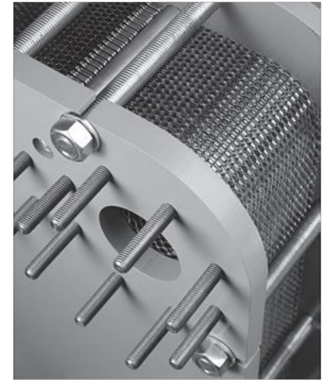
FIGURE 1.7 Plate heat exchanger. (a) Construction details—schematic (Parts details: 1, Fixed frame plate; 2, Top carrying bar; 3, Plate pack; 4, Bottom carrying bar; 5, Movable pressure plate; 6, Support column; 7, Fluids port; and 8, Tightening bolts.) and (b) closer view of assembled plates. (Courtesy of ITT STANDARD, Cheektowaga, NY.)
