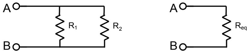
Figura 3:  $R_{eq} = \frac{R_1 R_2}{R_1 + R_2}$
