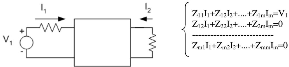
$$\begin{cases} Z_{11}I_1 + Z_{12}I_2 + \dots + Z_{1m}I_m = V_1 \\ Z_{12}I_1 + Z_{22}I_2 + \dots + Z_{2m}I_m = 0 \\ \dots \\ Z_{m1}I_1 + Z_{m2}I_2 + \dots + Z_{mm}I_m = 0 \end{cases}$$
