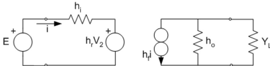
$$E = h_i i + h_r \left( -\frac{h_f i}{h_o + Y_L} \right) \Rightarrow Z_i = h_i - \frac{h_r h_f}{h_o + Y_L}$$
