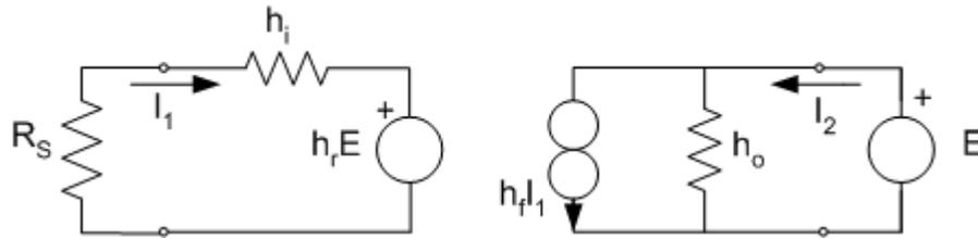
$$I = h_o E + h_f \left( -\frac{h_r E}{h_i + R_s} \right) \Rightarrow Y_o = h_o - \frac{h_r h_f}{h_i + R_s}$$
