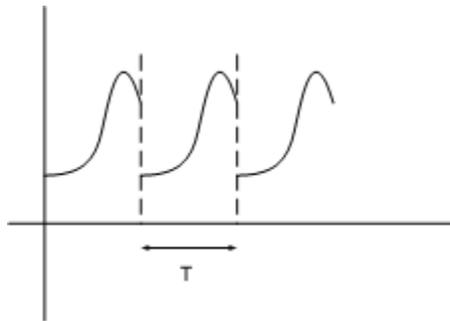
$$F(s) = \int_0^{\infty} e^{-st} f(t) dt = \int_0^T + \int_T^{2T} + \dots = \sum_{n=0}^{\infty} \int_{nT}^{(n+1)T} e^{-st} f(t) dt = (*)$$
