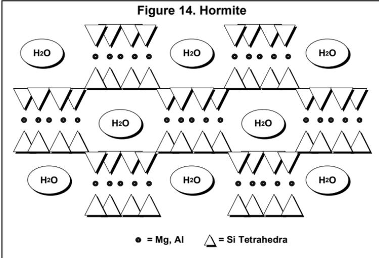
In addition to their use as absorbents, hormite clays are used as rheological agents. When dispersed in water, their needle-like particles deagglomerate in proportion to the amount of energy applied and form a random colloidal lattice.
